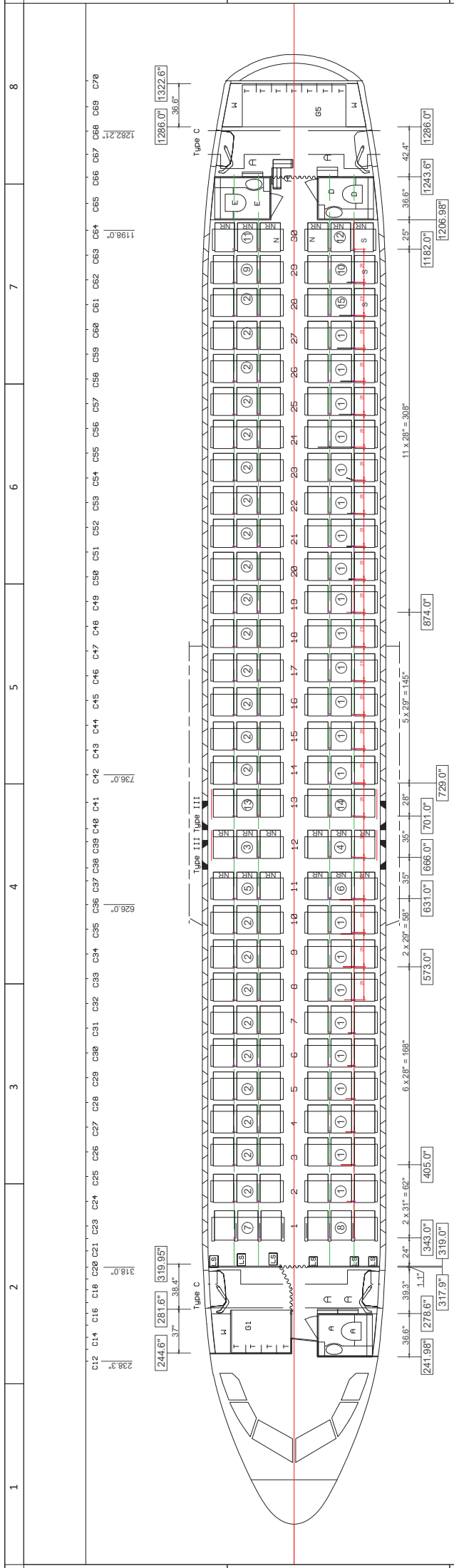
FIGURE 2-E1. LAYOUT OF PASSENGER ACCOMMODATIONS
